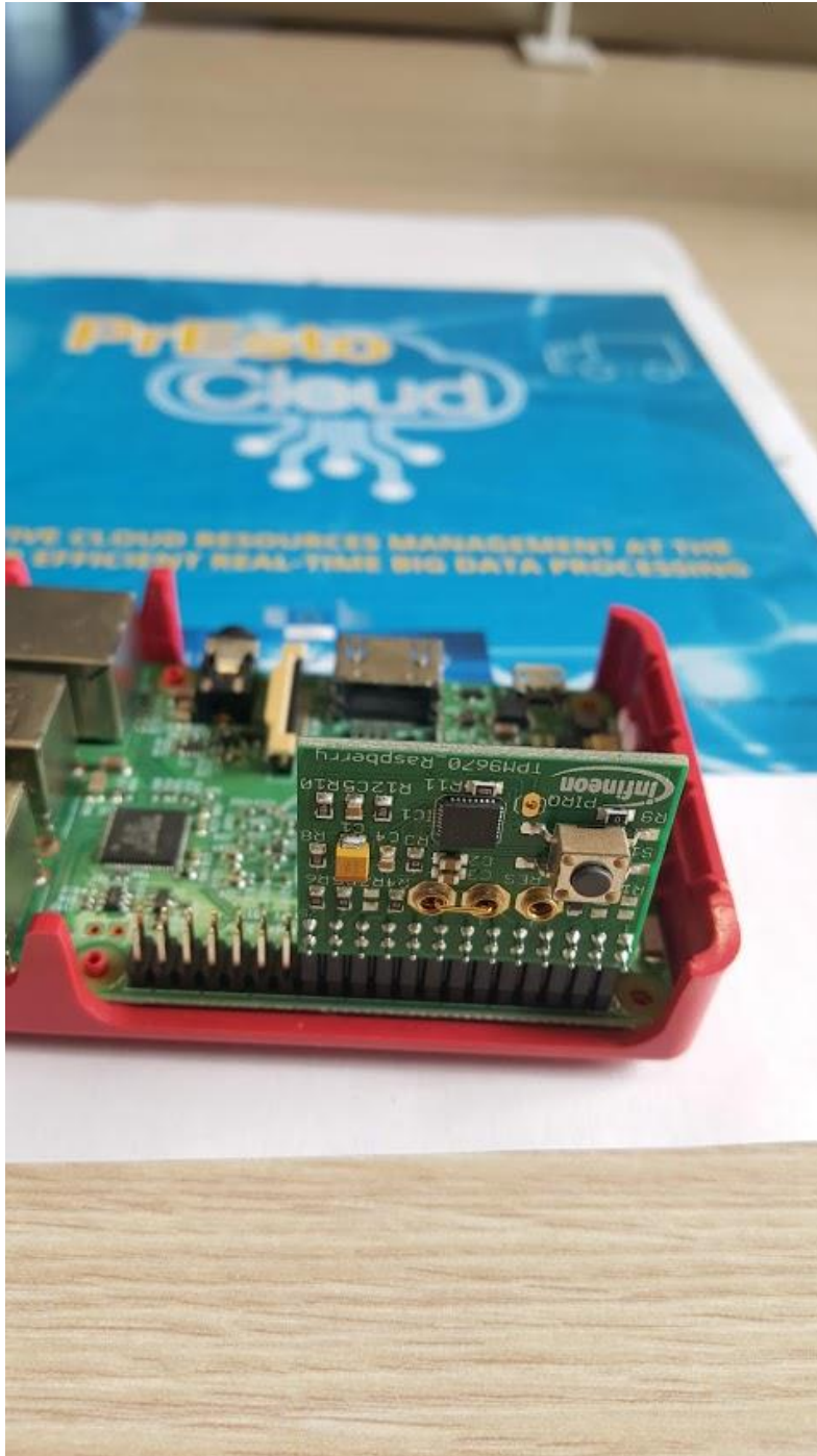
Figure 2 PrEstoCloud TPM testbed based on Infineon module on a Raspberry device
