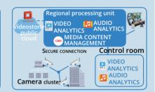
A surveillance solution combines real-time data streams from cameras and pre-processing results from groups of unmanned aerial vehicles.
